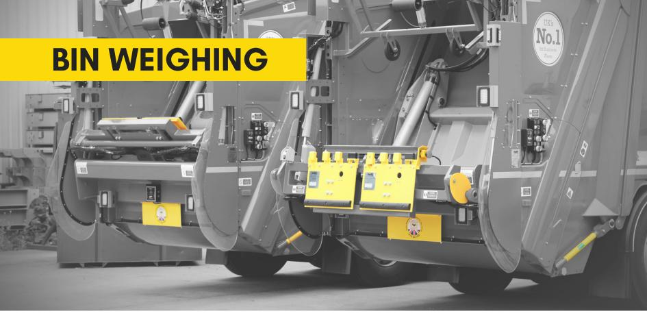
ENVIROWEIGH is a trade certifiable dynamic bin weighing system - accurate to class Y (b). It can be installed onto most types of RCVs lifting hoists and weighs the precise weight of waste collected from wheeled bin containers during the normal loading cycle. There is no need to stop the lifter and speeds are not compromised. Each lifting chair is installed with a weighing load cell and can weigh two bins independently and simultaneously.
